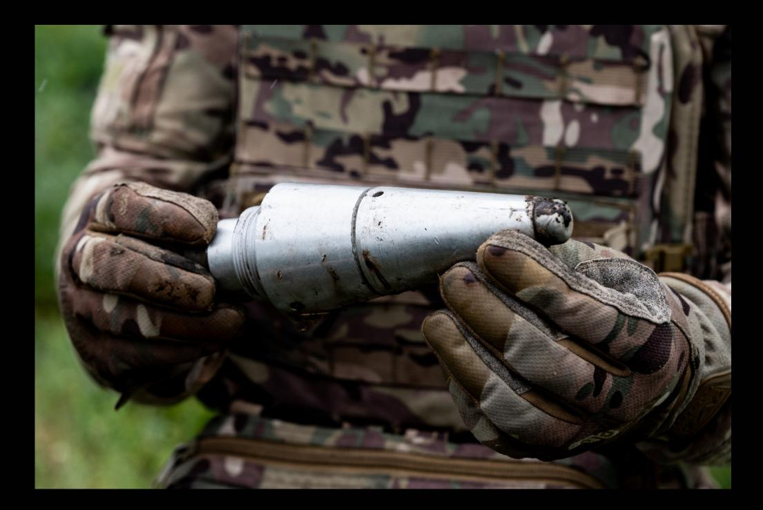
Kherson Oblast (exact location not disclosed) - The fuse from a 152mm howitzer shell after it has been removed from a live shell.
